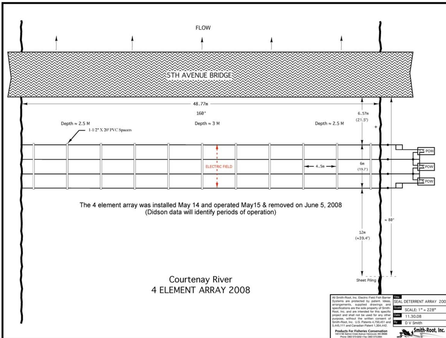
Figure 3. Schematic of the 4-cable array tested in the Courtenay River upstream of the 5<sup>th</sup> Street bridge between May 14 and June 5, 2008.
