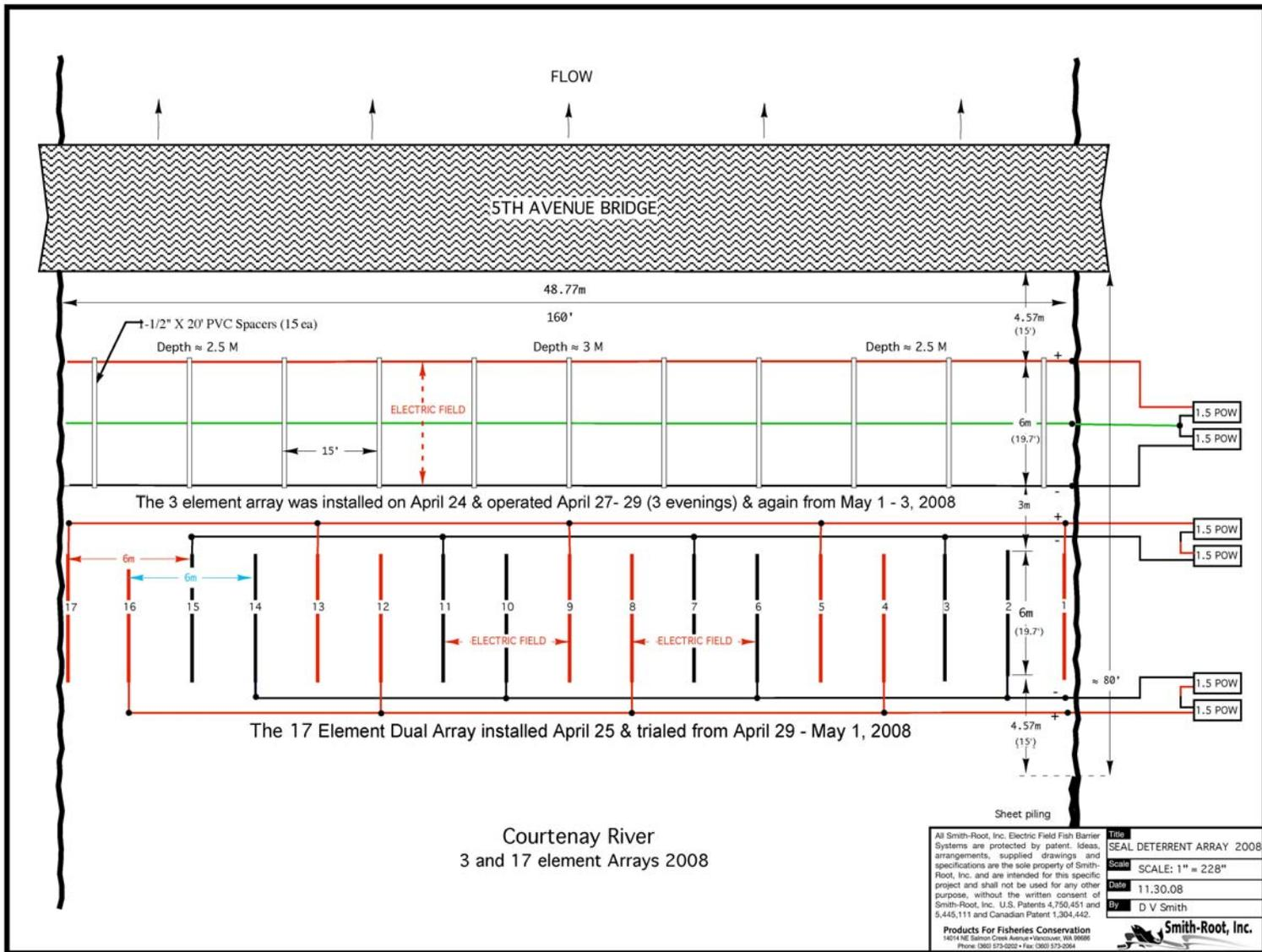
Figure 2. Schematic of the 3-cable and the 17-element arrays tested in the Courtenay River upstream of the 5<sup>th</sup> Street bridge between April 27 and May 3, 2008.
